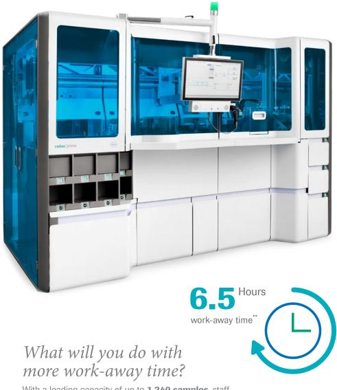
With a loading capacity of up to **1,240 samples**, staff can achieve up to 6.5 hours of work-away time that can be devoted to other testing priorities while routine testing automatically proceeds in the background.\*\*
